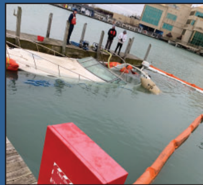
Pollution responders oversee a response as boom is placed to contain the fuel leak from a sunken recreational vessel
